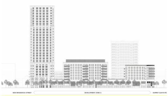
**Image above:** Proposed Park Walk Elevation showing Block C, Block B and Block A with Block D in the background
