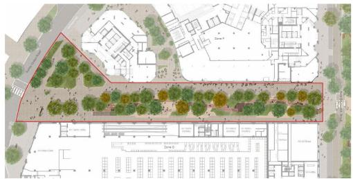
**Image above:** Park Walk layout with Plot F to the north and Plot G to the south – the space comprises a central landscaped route with shared pedestrian and cycle routes on either side
