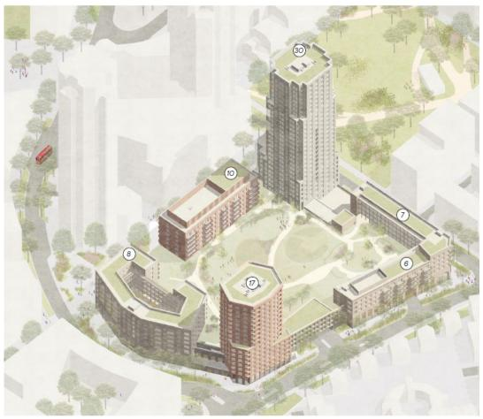
**Image above:** Site diagram showing the arrangement of five blocks above the 3 storey podium supermarket and car park with storeys annotated
