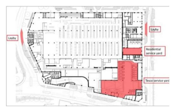
**Image above:** Proposed layout showing key service areas and vehicular entry/exit points
